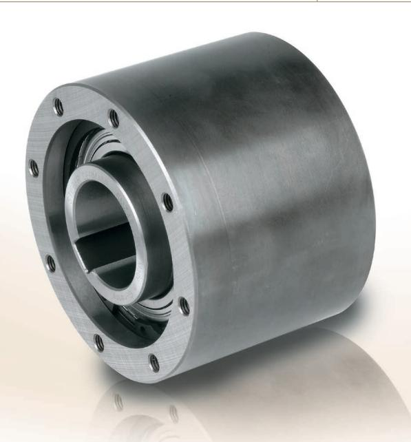
ype SMZ is a sealed, sprag type freewheel, bearing supported using two 60..ZZ series grease lubricated bearings.
