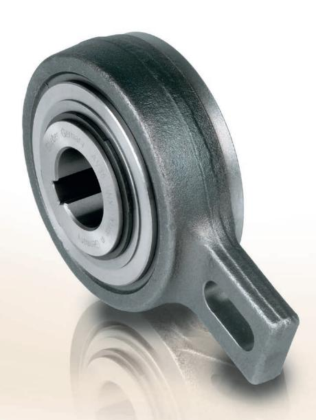
ype AV is a roller type freewheel. It is self-contained, centered by plain bearings for low rotational speeds, and sealed using shield protected metallic labyrinth seals
