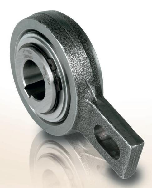
ype RSBW is a DC sprag type freewheel. It is self-contained, centered by plain bearings for low rotational speeds and sealed using shield protected O Rings.
